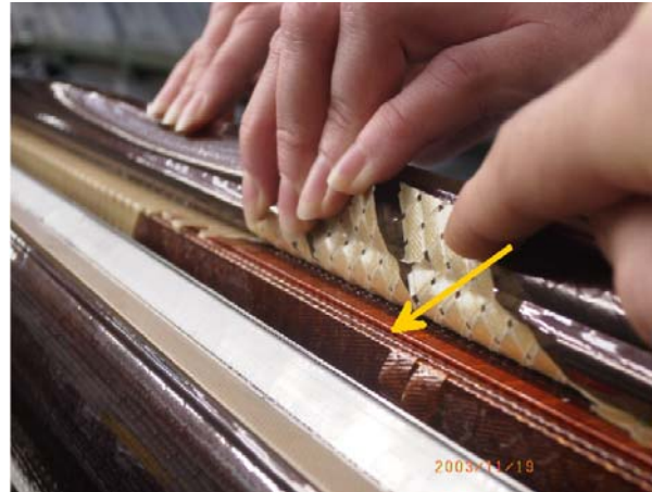
Fig. 22. A case of bad coil curing giving a inner radial movement of two turns of the inner layer, upper pole, of about 1 mm, found through anomalies in room temperature magnetic measurements.
