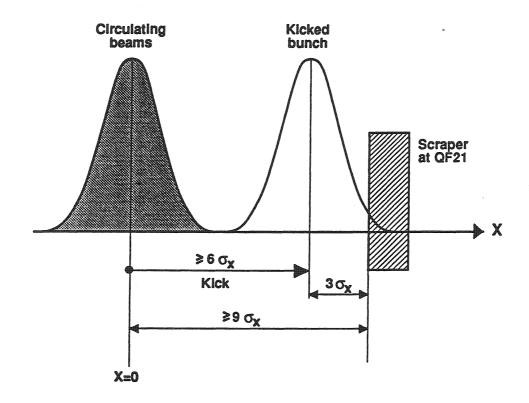
Figure 27.1: Bunch intensity equalisation with the injection kicker system
