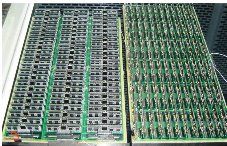
Figure 5.8: Photographs of two types of PMD modules showing the boundary frames and the connectors with the FEE boards mounted.
