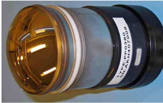
Figure 6.7: Left: a schematic and right: a photograph of the pixel-HPD.
