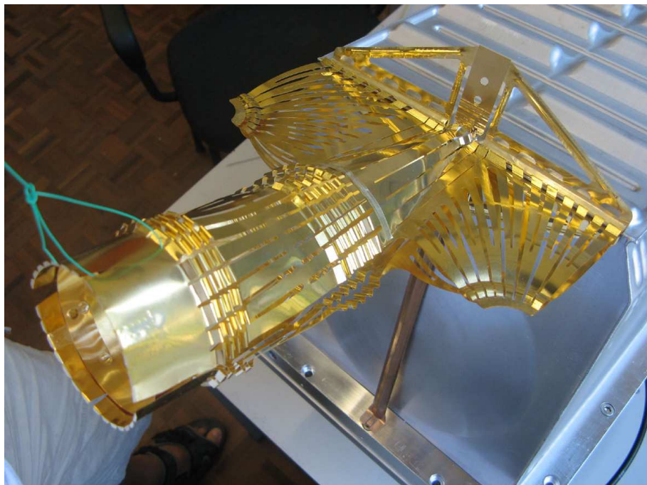
Figure 5.9: Photograph of the downstream wakefield suppressor.
