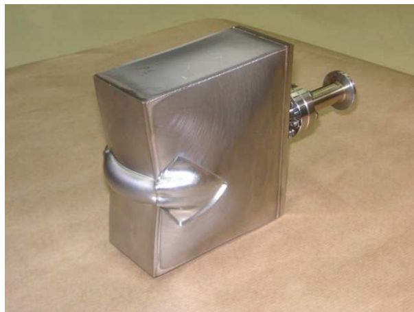
Figure 4.6: Deformation of the thin window after the ultimate pressure test, stopped at 80 bar.
