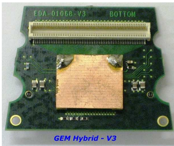
Figure 5.18: The TOTEM gas detector hybrid carrying one VFAT readout chip (under the cover).
