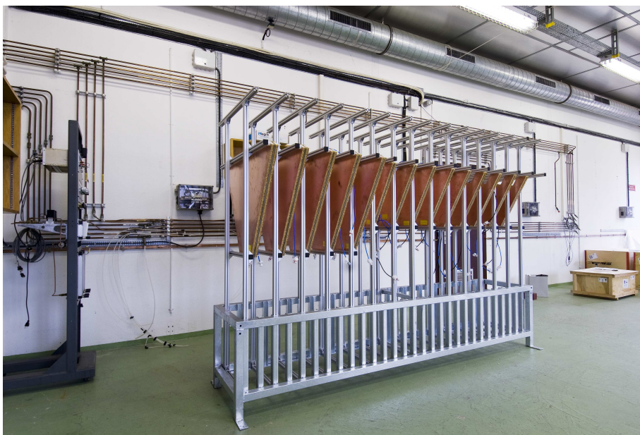
Figure 5.7: Completed CSC chambers for T1 in a test area at CERN.
