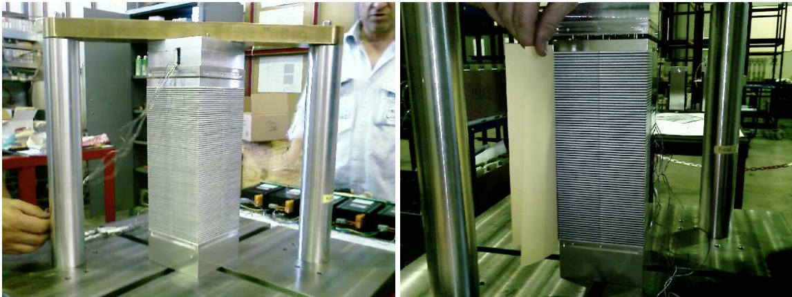
Figure 2.9: Left: Assembled module on the assembly station after removing the stacking fixture, and with the load cells and the crossbeam installed. Right: The module during the installation of the black light-blocking foil.
