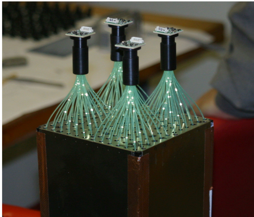
Figure 2.12: Fiber bundles with attached APD and preamplifier of four towers of an EMCal prototype module.
