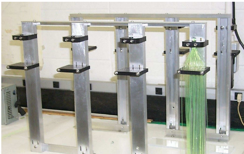
Figure 2.7: A fixture used to position the WLS fibers into the correct convergent shape that transitions from the uniform sampling of the tower volume to the small circular diameter required to mate to the light guide/diffuser.
