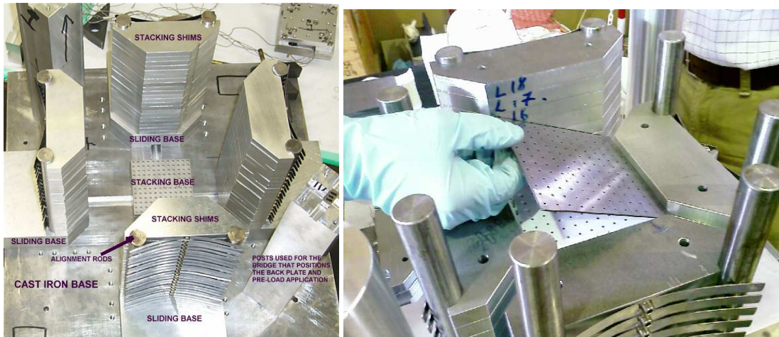
Figure 2.8: Left: Stacking fixture prior to the insertion of any EMCal components. Right: Stacking fixture during the assembly of a prototype module.
