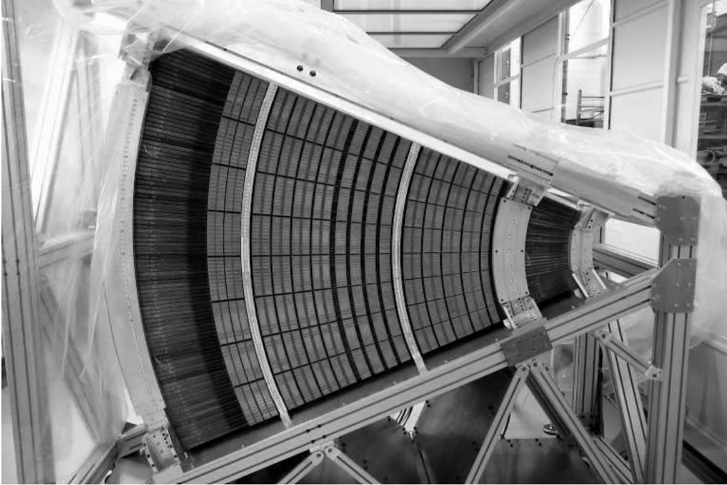
Figure 4. Front view of the first EMEC module, after completion of the stacking, showing some structural elements (the module is held by the stacking frame). All summing boards, except one type (at largest radius), are plugged to the electrodes.
