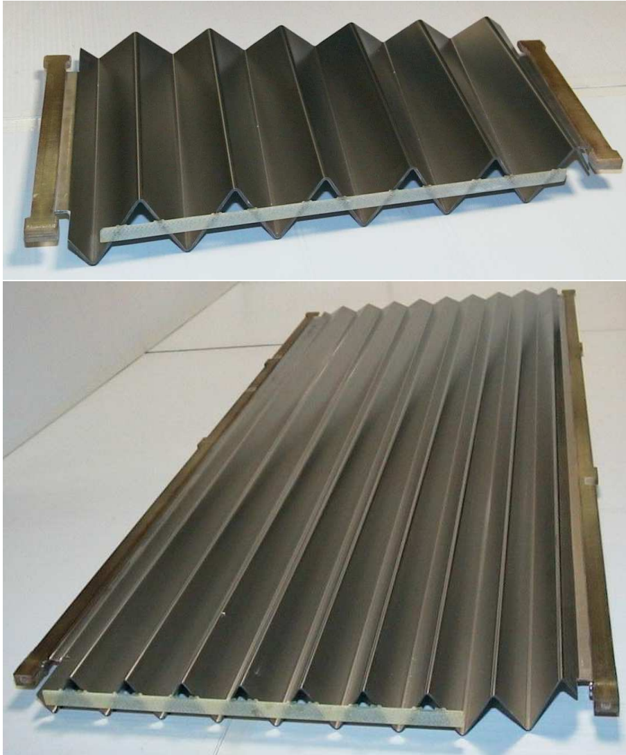
Figure 10. Small (top) and large (bottom) absorbers. On each absorber, the longitudinal bars parallel to the waves and the transversal bar glued on the waves are clearly visible.
