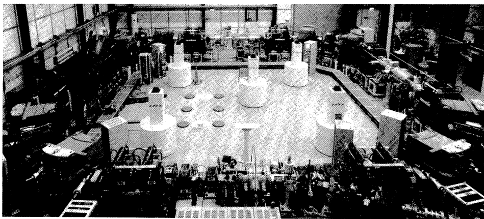
FIGURE 1 The Heidelberg Test Storage Ring for Heavy Ions TSR. The Electron Cooler can be seen in the left straight section.
