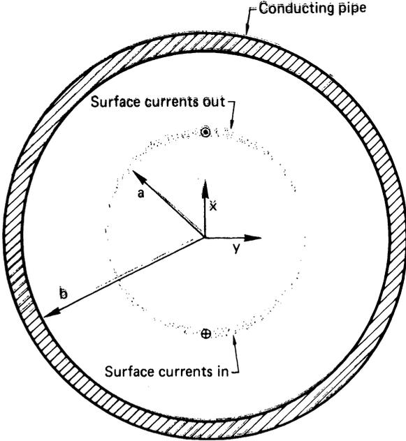
FIGURE 1 Equivalent surface charge and current density layers of beam displaced from the axis of a conducting pipe.
