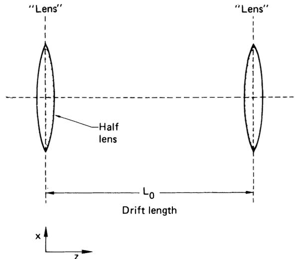
FIGURE 4 A single half-lens drift length half-lens combination.
