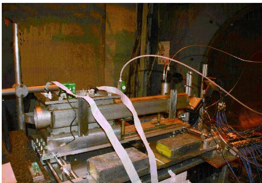
Figure 79. FP420 2007 test beam setup including one movable station, two blades, and two timing detectors (one GASTOF and two QUARTICS).
