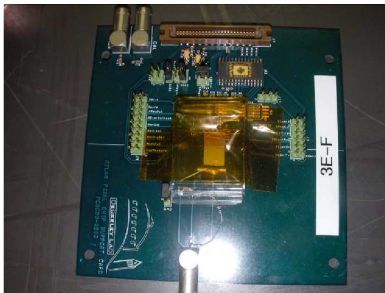
Figure 75. Picture of the 3D-ATLAS pixel assemblies mounted on one of a pcb testboard with a protective cover.
