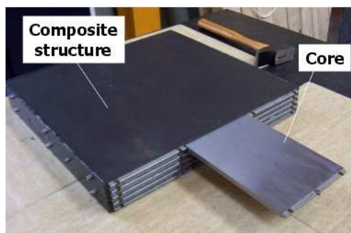
Figure 4. Moulding of an alveolar structure: metal cores alternate with tungsten, both wrapped in carbon fibre-epoxy composite.
