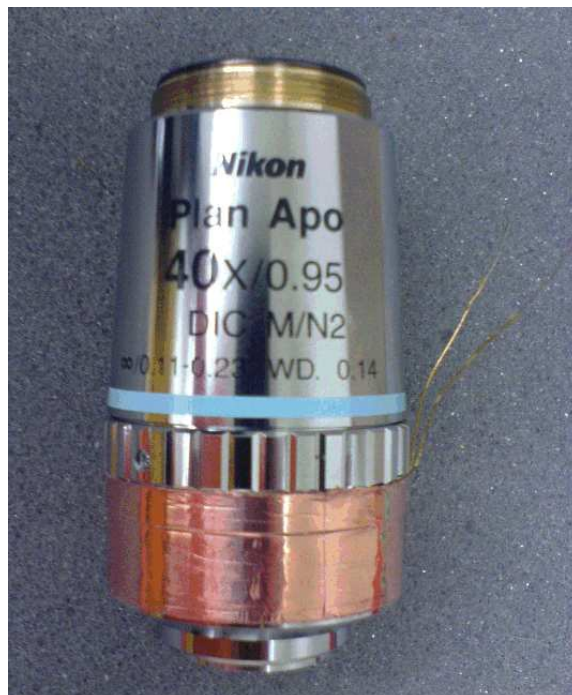
Figure 10. NIKON Plan Apochromat dry objective lens, \times 40 magnification, N.A. = 0.95 , with cover glass correction collar and heating coil.
