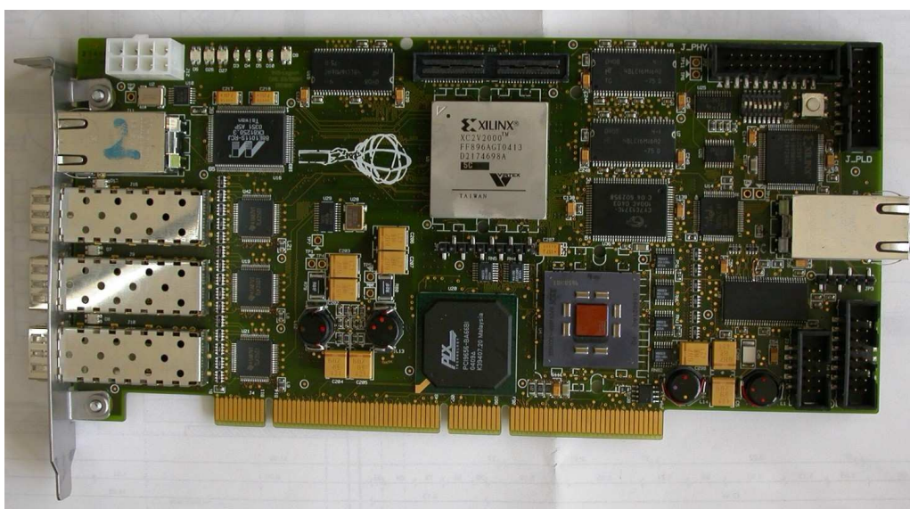
Figure 4. The ROBIN card. The connectors at the left (from top to bottom) are for Gigabit Ethernet (electrical connection) and for three HOLA S-links (optical). The FPGA is at the center of the board (part labelled with "Xilinx"), the chip below it is the PCI bus interface, immediately right of the PCI interface the PowerPC 440 microcontroller can be seen. The connector at the right is for the 100 Mbit Ethernet connection of the PowerPC. The left connector of the pair of connectors at the lower right corner of the board provides an RS-232 connection to the microcontroller. Just above the FPGA is a connector for a mezzanine board.
