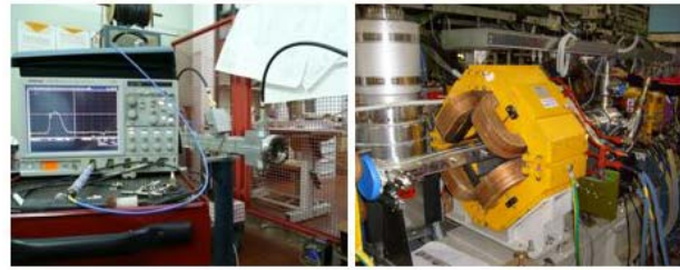
Figure 7: New fast injection kicker under test (left) and installed on the electron ring (right).
