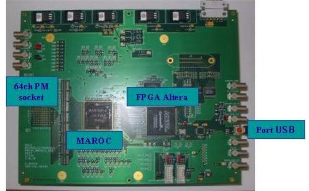
Figure 4: Picture of the test board used for characterisation tests.
