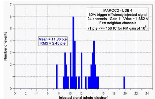
Figure 14: Injected signal for which cross-talk appears.
