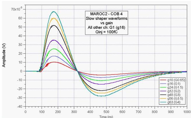
Figure 12: Slow shaper waveforms for a fixed injected charge of 100 fC and seven different preamplifier gains.
