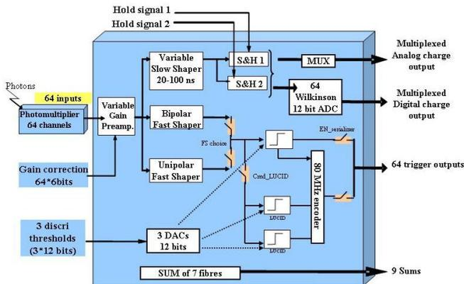
Figure 3: Block diagram of MAROC second version.
