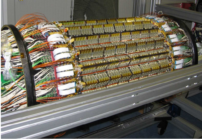
Figure 6: The SDD detector completely assembled, ready to be integrated with the Silicon Strips.
