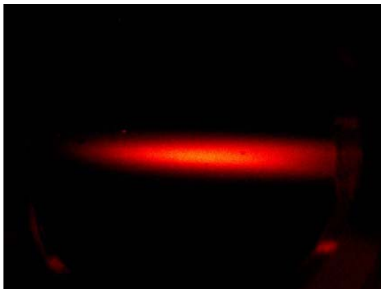
Fig. 35a: Electron beam image on screen 1, solenoid switched off.
