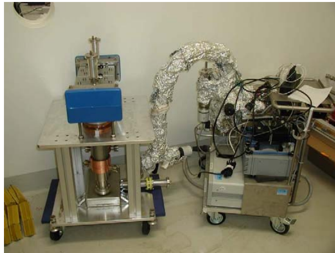
Fig. 11: Conditioning of the 10 kW main power coupler
