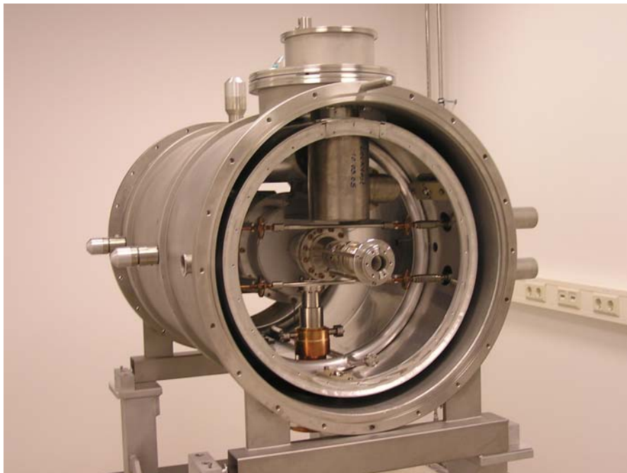
Fig. 4: Photograph of the cryostat vessel during assembly.
