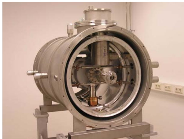
Assembly of the SRF gun cryomodule at FZD
