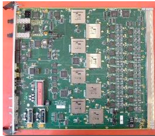
Figure 18: Photograph of a CPM. From right to left, de-serialiser and serialiser chips, 8 CP chips, optical readout to DAQ and L2.
