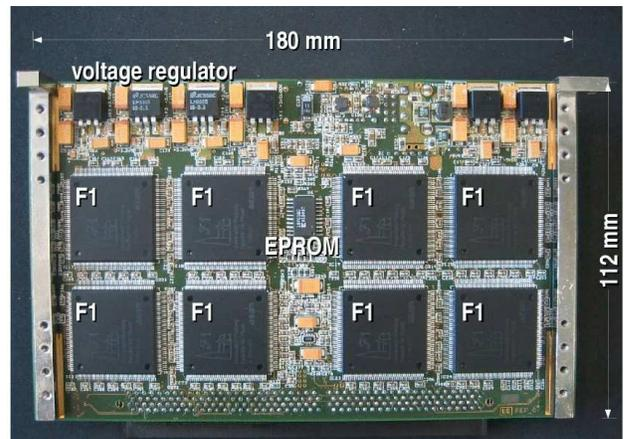
Fig. 5. Front side of the DREISAM card with 8 F1-TDC chips.
