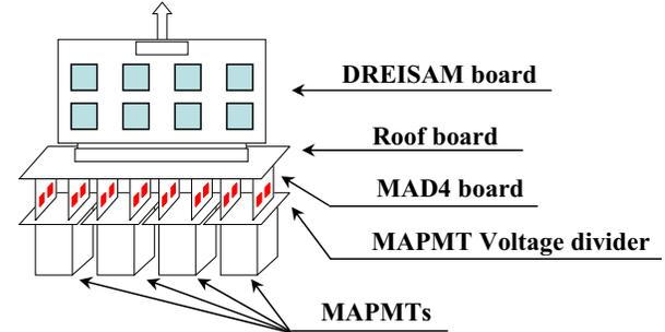
Fig. 1. Scheme of the read-out system.
