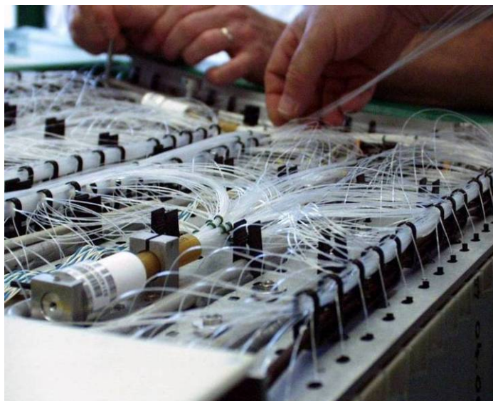
Figure 10. The ECAL barrel tertiary (L1) fan-out and its diffusing sphere assembly shown installed on a SM front face.
