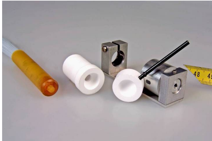
Figure 9. The ECAL barrel tertiary (L1) 240-fiber optical fan-out assembly. The fan-out inserts into a 12 mm I.D. diffusing sphere (shown opened here). Light is injected at 90° to the fan-out's axis via the ferrule.
