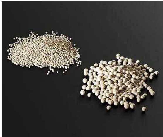
Figure 7: Zeolite Beads UY8
