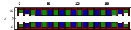
Fig. 2 Short version of the proposed wiggler with a gap of 5 mm and a period length of 2.1 cm. Green and blue are superconductive wire bundles. The different colors mark different current directions. The corresponding field is shown in Fig. 3.
