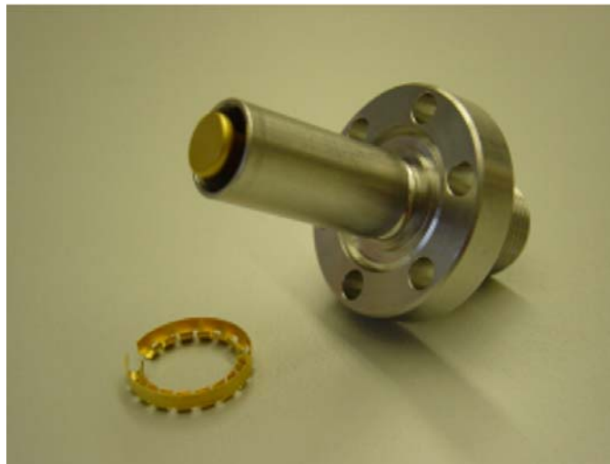
Fig. 15 Button electrode from the Tesla Test Facility at DESY (courtesy D. Noelle and M. Wendt, 2003).
