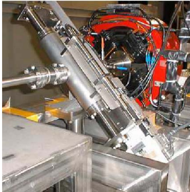
Fig. 41 Wire scanner assembly in the extraction line of the ATF damping ring (courtesy H. Hayano, 2003).
