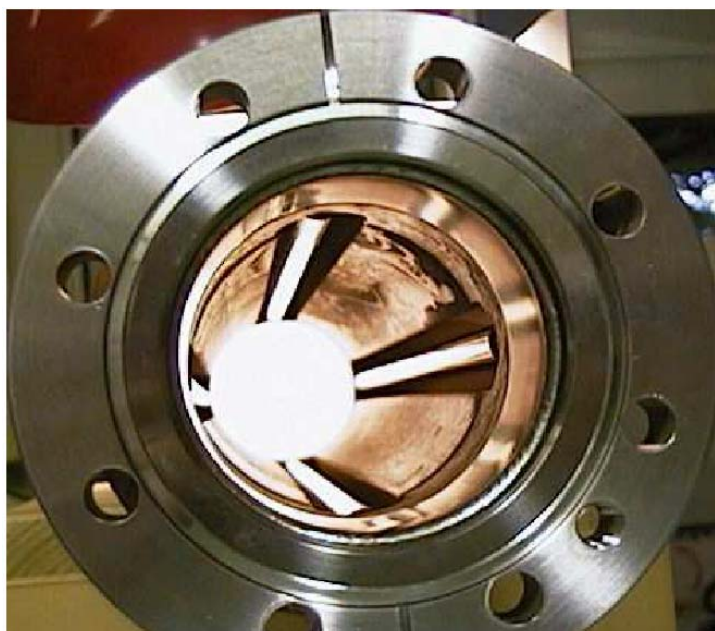
Fig. 18 Photograph of a stripline BPM from the HERA accelerator at DESY (courtesy M. Wendt, 2004).
