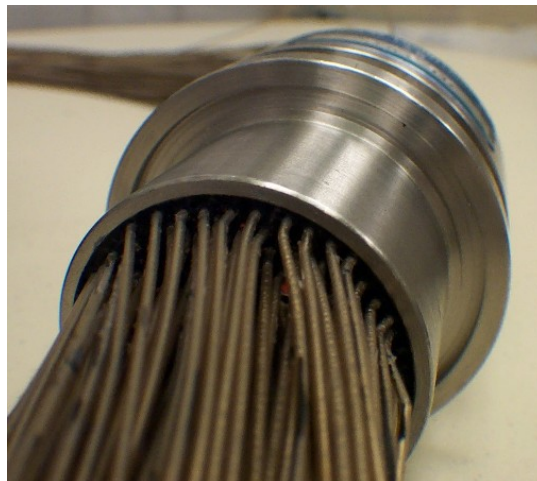
Figure 8. An illustration of Wire Feedthrough faults (left). Right: wires exiting a WFT on the cold side, showing the high-density 216-wire HV bundle.
