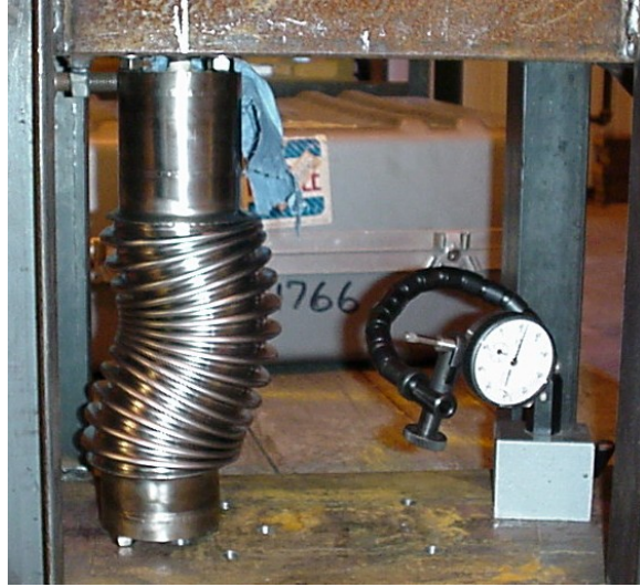
Figure 4. “Squirm” test of a bellows unit. Squirm occurred at 190 psi (13 atm).
