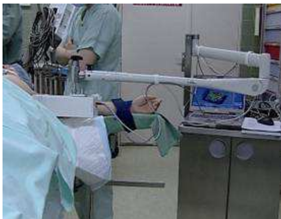
Figure 15. Picture of the mini gamma camera on its support.
