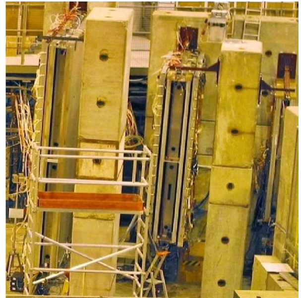
Fig. 17.8: Displacement of the various coils while 21 kA were put in the toroid
