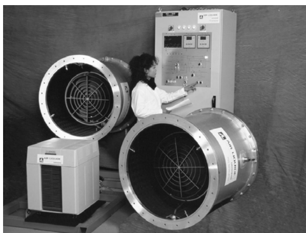
Fig. 16: Large cryopump for space simulation chambers
