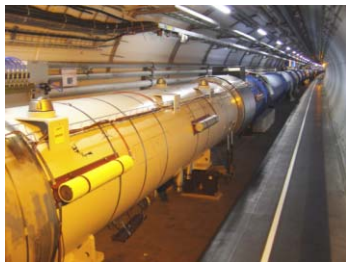
Figure 1: The LHC beam loss monitors (yellow insulation, mounted on a red support) are mounted on the outside of the cryostats, horizontally aligned to the beam pipe.
