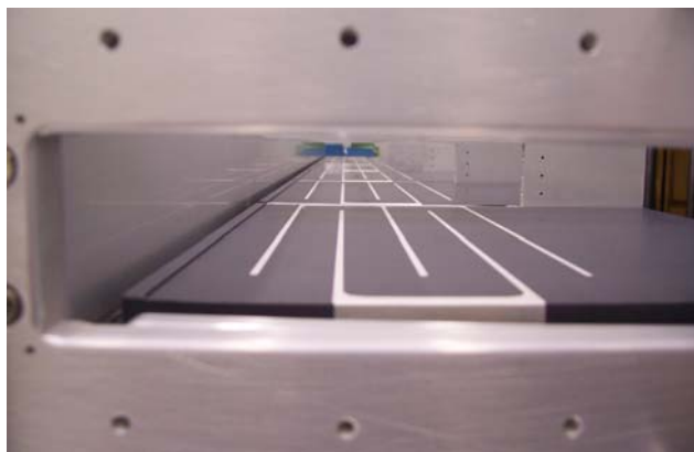
Figure 4. Metallic stripes applied to SPS extraction kicker ferrites, for impedance reduction purposes.
