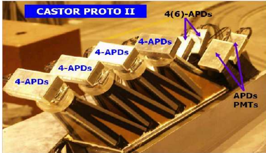
Figure 4: Assembled prototype II on the moving table in the CERN/SPS H2 beam line. Only the APD readout units are shown.
