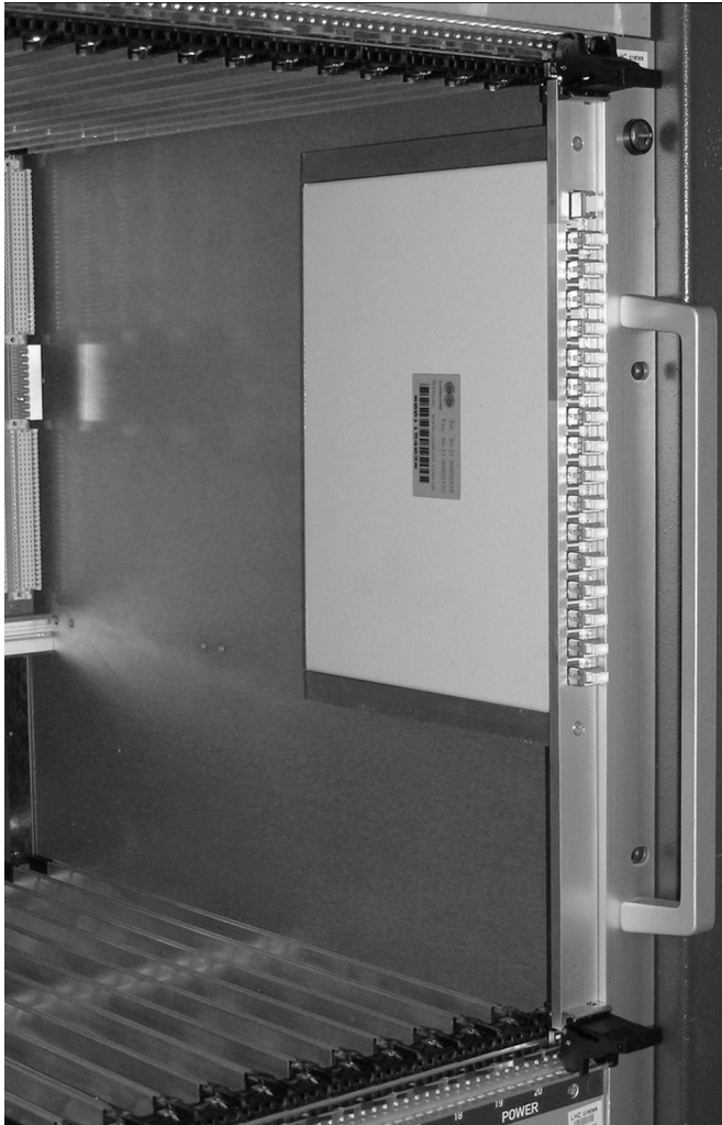
Fig. 4. 1 \times 16 Optical Splitter mounted in 9U VME crate. The input is at the top, with 16 outputs below. A 9U front-panel supports the card in the VME crate.
