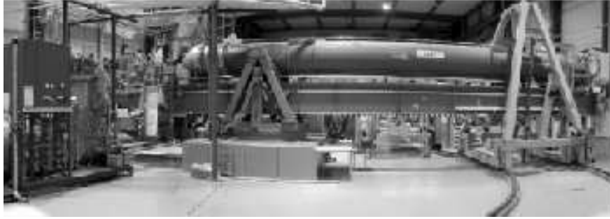
Fig. 5. Experimental setup of the CAST experiment at CERN. From the left to the right the Helium cryogenic system, the CAST superconducting magnet, and the tracking system is shown. The tracking system allows to follow the Sun 1.5h per day during sunrise and sunset
