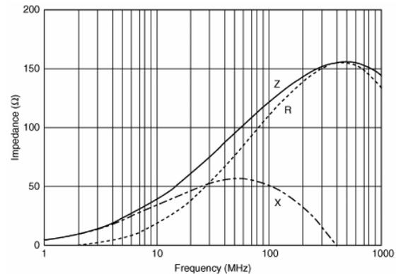
Figure 4: Impedance-frequency characteristics of BLM18PG121 ferrite, from Murata.
