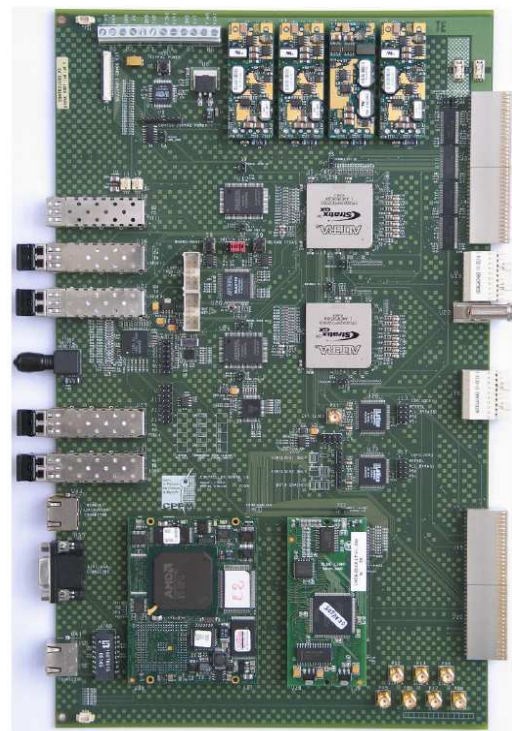
Figure 10: Top view of the controller board.
