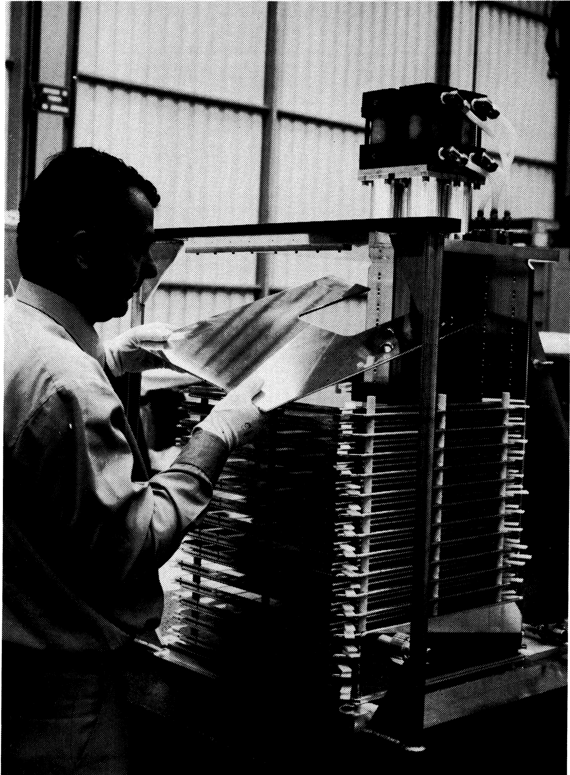
Fig. 4 Assembly of a magnet module.
