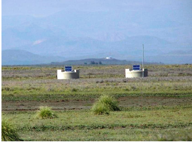
Fig. 10: The detector pair of the Engineering Array, Carmen and Miranda, used for estimating the timing accuracy with which signals are recorded at the detectors. Signal size accuracy is also determined from such pairs, of which there are two on the production array. The Los Leones fluorescence site is visible in the distance between the detectors.
