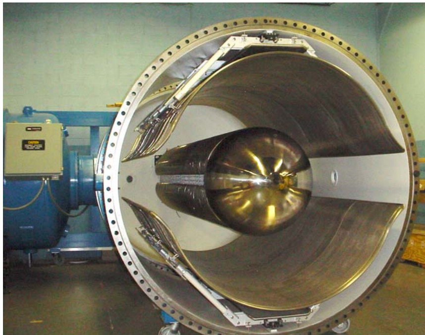
Fig. 20: Photograph of a 5 MV Dynamitron accelerator. From Radiation Dynamics, Inc.
