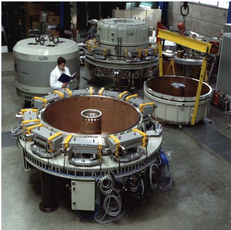
Fig. 24: A photograph of an IBA Rhodotron being assembled in Belgium. From Ion Beam Applications.
