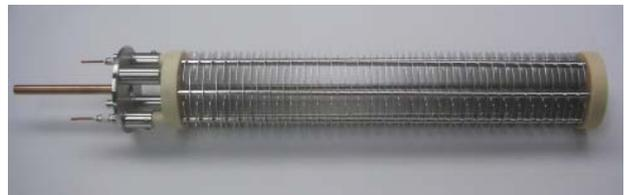
Fig. 2. Inside structure of the LHC BLM (ionization chamber).
