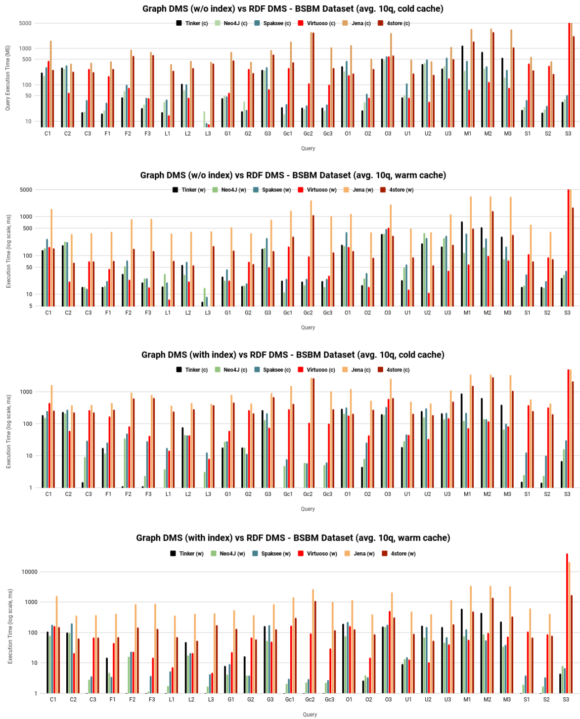
Figure 5.7: Performance comparison of SPARQL queries vs the translated Gremlin traversals for BSBM dataset with respect to RDF and Graph DMSs in different configuration settings.
