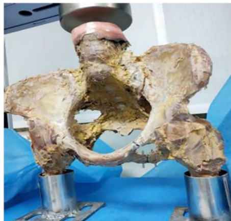
Fig. 3 Tile B fracture cadaver model, each left superior ramus and the inferior ramus of the pubis-ischium was sawed vertically
