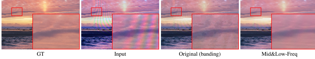
Figure 5: Visualization of results under different calibration strategies. Original: training in the spatial domain suffers from banding artifacts under low-bit quantization. Mid&Low-Freq: our frequency-aware calibration strategy leverages mid- and low-frequency to mitigate banding.
