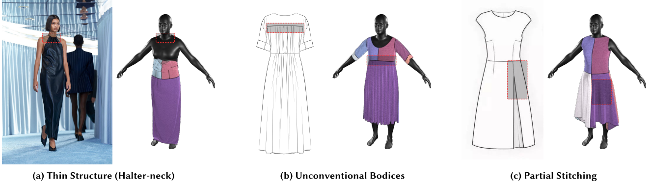
Figure 14. Limitations of Design2GarmentCode, including failed to modeling thin structures like halter-neck, unable to model unconventional bodices and stitching relationships are limited to one-to-one mapping.
