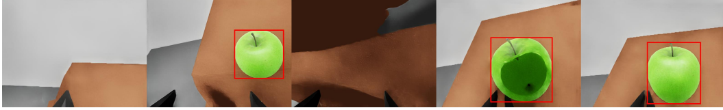
Figure 11: An example of IK failure (view of the left camera): the object is at the edge of the robotic arm’s workspace - a case where the object height is too low.
