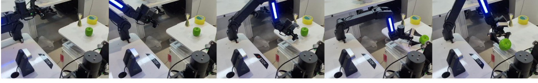
Figure 14: Task: Cluttered Table. Grasp the apple from a cluttered table with a height of 60 cm.
