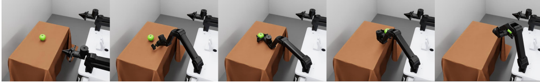
Figure 21: The simulation environment consists of a room with a table, an apple, and a robot. The task is for the robot to grasp the apple and place it in a specified location.
