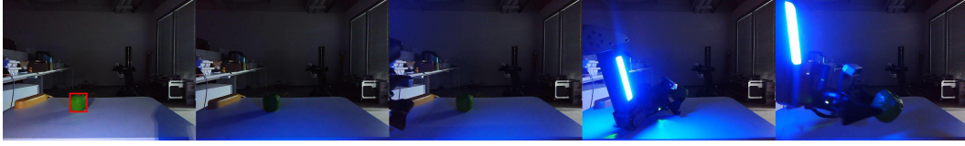
Figure 7: A case of detection failure. The task is to catch apples at a specified location in a fluttering light environment.
