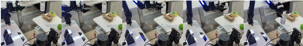
Figure 13: Task: Mid-Air. Grasp the bottle lifted by hand and suspended in mid-air, then move it to the target position.
