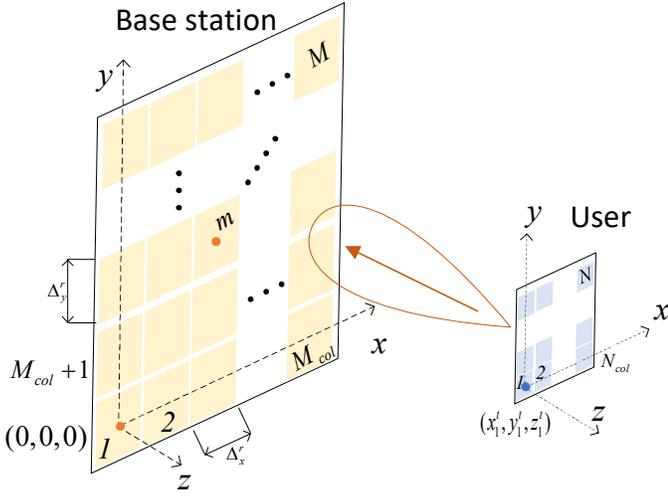
Fig. 1: Illustration of antenna patches and their coordinates.
