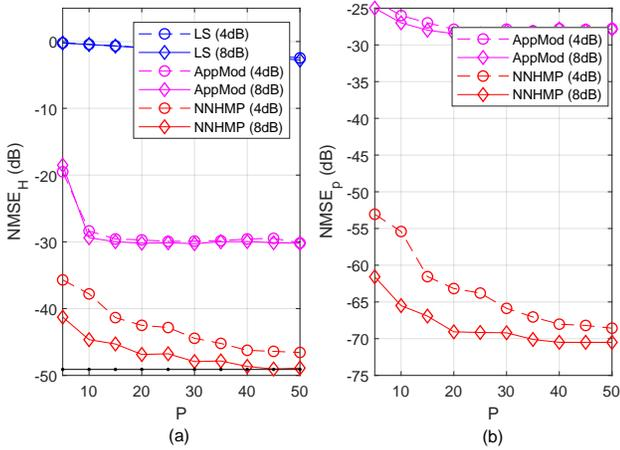
Fig. 12: NMSE of the estimators with hybrid receiver versus  $P$ .
