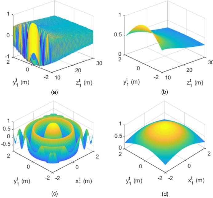
Fig. 2: The real part of  $h_{11}^{xx}$  (a) and (c) and the real part of  $h_{11}^{xx}/\exp(ik_0 r_{11})$  (b) and (d).
