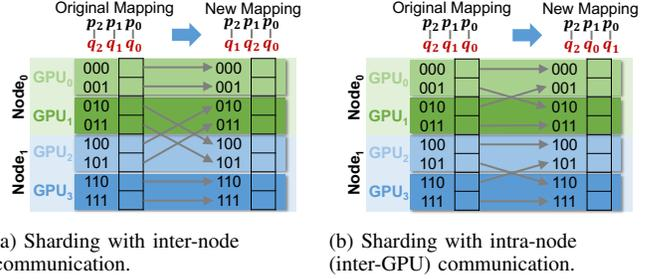
Fig. 2: Sharding with different types of communication. The simulation has 1 local, 1 regional, and 1 global qubit.  $p_i - q_j$  indicates that the  $i$ -th physical qubit is mapped to the  $j$ -th logical qubit. Inter-node communication is triggered if we update any global qubits (Figure 2a), and only intra-node communication is triggered otherwise (Figure 2b).
