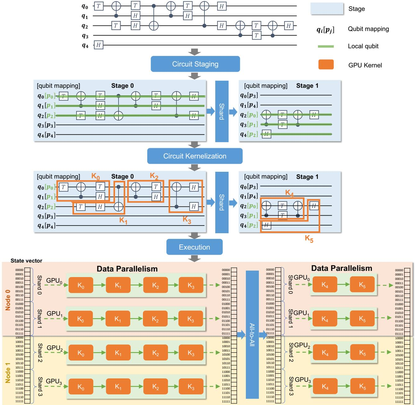
Fig. 1: An example application of circuit partitioning and execution. We stage the circuit so that qubits of each gate map to local qubits (i.e., green lines in each stage). The notation  $q_i[p_j]$  indicates that the  $i$ -th logical qubit maps to the  $j$ -th physical qubit. The KERNELIZE algorithm then partitions the gates of each stage into kernels that provide for data parallelism.
