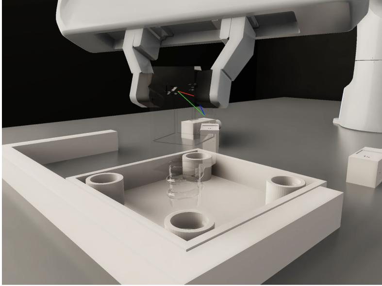
Figure 11: Visualization of the effect of the residual policy during insertion, the phase requiring the most precision. The red line shows the action commanded by the base policy. The blue is the correction predicted by the residual, and the green is the net action. The residual learns to correct actions that typically lead to failure.
