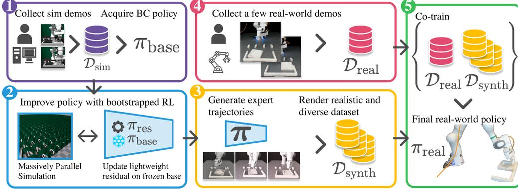
Figure 1: **Pipeline overview.** (1) Beginning with a policy trained with BC in simulation, (2) we train residual policies to improve task success rates with RL and sparse rewards. (3) We then distill the resulting behaviors to a policy that operates on RGB images. (4) By combining synthetic data with a small set of real-world demonstrations, (5) we deploy assembly policies that operate from RGB images in the real world.
