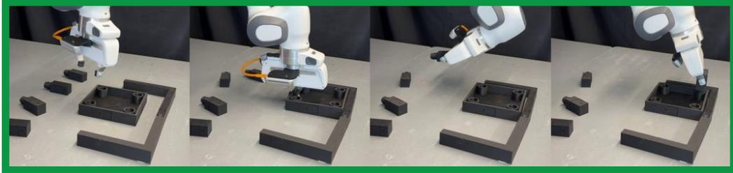
Figure 14: An example of a successful rollout of a policy co-trained on 40 real-world demos containing only white parts and 400 synthetic demos with part colors randomized.
