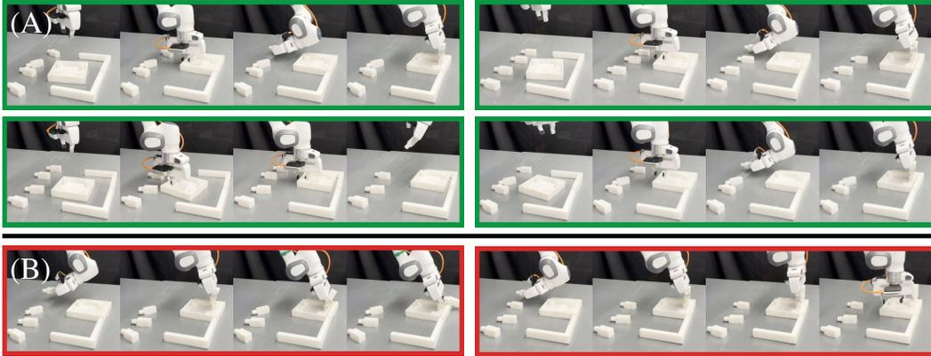
Figure 6: **(A)** Examples of successful real world assembly from RGB. Co-training with simulation data reduces jerkiness and improves insertion robustness, due to data from simulation containing higher diversity of initial part poses and insertion locations (see Table 2). **(B)** Representative failures, primarily due to overfitting to a particular corner location and difficulty adjusting the insertion angle/position when grasps lead to unfamiliar in-hand part poses.
