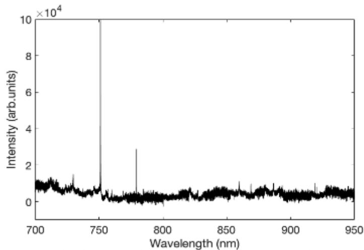
**Figure 4:** Composite Au spectrum obtained for the 700 – 950 nm range at a laser intensity on target of  $6 \times 10^8 \text{ Wcm}^{-2}$ . The quantum efficiency of our CCD camera limited the measurements to  $< 1000 \text{ nm}$ .
