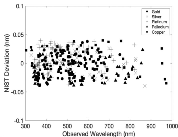
**Figure 2:** Plot of the differences between tabulated NIST wavelengths and our spectrometer measurements for relevant elements.
