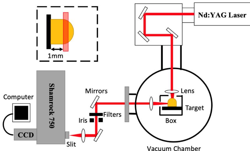
**Figure 1:** Top-view schematic of the experimental setup, with the Au target placed inside the vacuum chamber. An Andor Shamrock 750 spectrometer was coupled to an Andor iKon-M CCD camera which collected the Au spectral data. The inset shows the section of the Au plasma that was focused onto the slit of the spectrometer outside the vacuum chamber.
