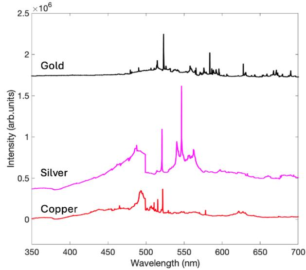
**Figure 5:** Experimental spectra of Au (99.95 % purity), Cu and Ag targets in the 350 – 700 nm range, obtained at a laser intensity of  $6 \times 10^8 \text{ Wcm}^{-2}$ . Spectra have been vertically displaced for ease of viewing.
