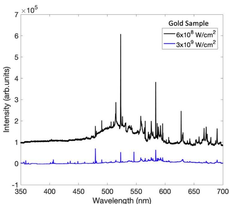
**Figure 3:** Composite Au spectra covering 350 – 700 nm recorded at two different laser intensities. The focal spot diameters of the black and red spectra were 3 mm and 1.3 mm, respectively, for a fixed laser energy of 400 mJ. The vacuum chamber window is 10 mm BK7 glass and so transmission starts to drop at wavelength below 400 nm. Spectra have been vertically displaced for ease of viewing.
