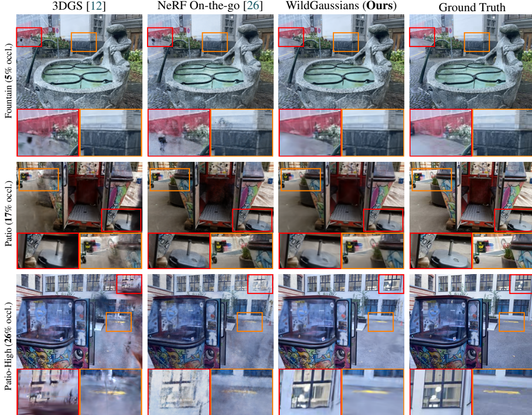
Figure 4: Comparison on NeRF On-the-go Dataset [26] . For both the Fountain and Patio-High scenes, we can see that the baseline methods exhibit different levels of artifacts in the rendering, while our method removes all occluders and shows the best view synthesis results.
